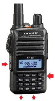
Turn on the radio by turning the volume knob clockwise until the radio turns on.
